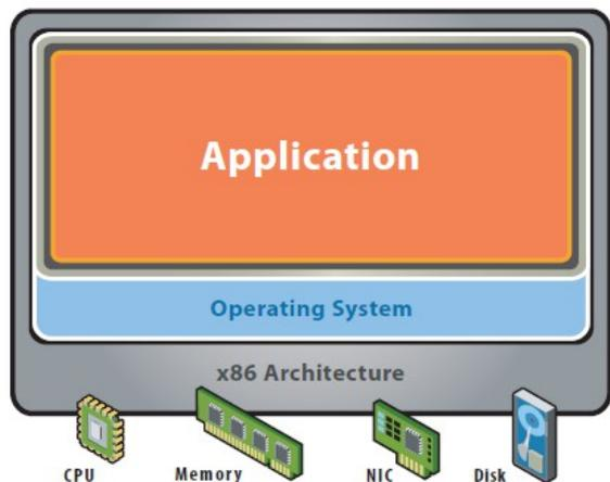
Fig.1. x86 Architecture before Virtualization [2]
