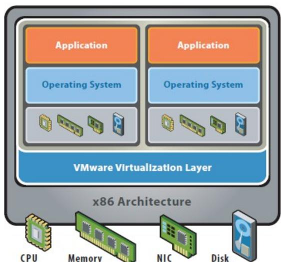
Fig.2. x86 Architecture after Virtualization [2]
