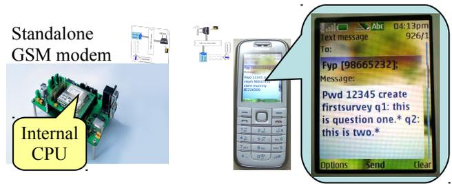
Fig. 2. Physical configuration of in-built application using GSM modems
