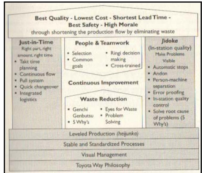
Figure 1. The Lean Manufacturing (Toyota Production System (TPS)). Source: Ref. [2] page 33.
